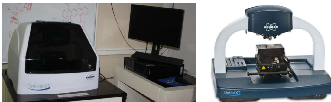
Figure 3.16 : DektakXT stylus profiler at IIT Jodhpur, used to measure the film thickness of spectrally selective absorber coatings in the present study.
