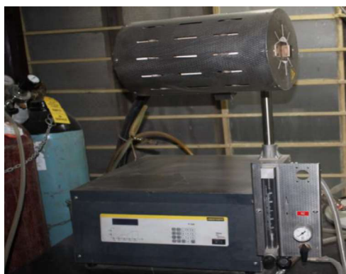
Figure 3.9 : Tabular furnace (Nabertherm GmbH) in our lab used for annealing of spectrally selective absorber films in this study.
