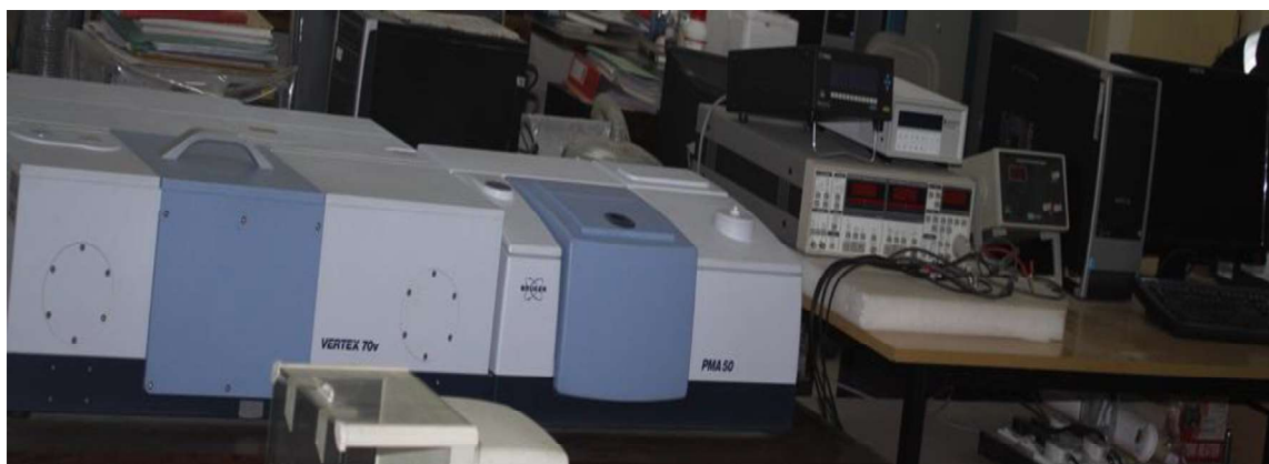
Figure 3.19 : Bruker FTIR spectrometer vertex 70v in our lab used to collect the reflectance spectra of spectrally selective absorbers.
