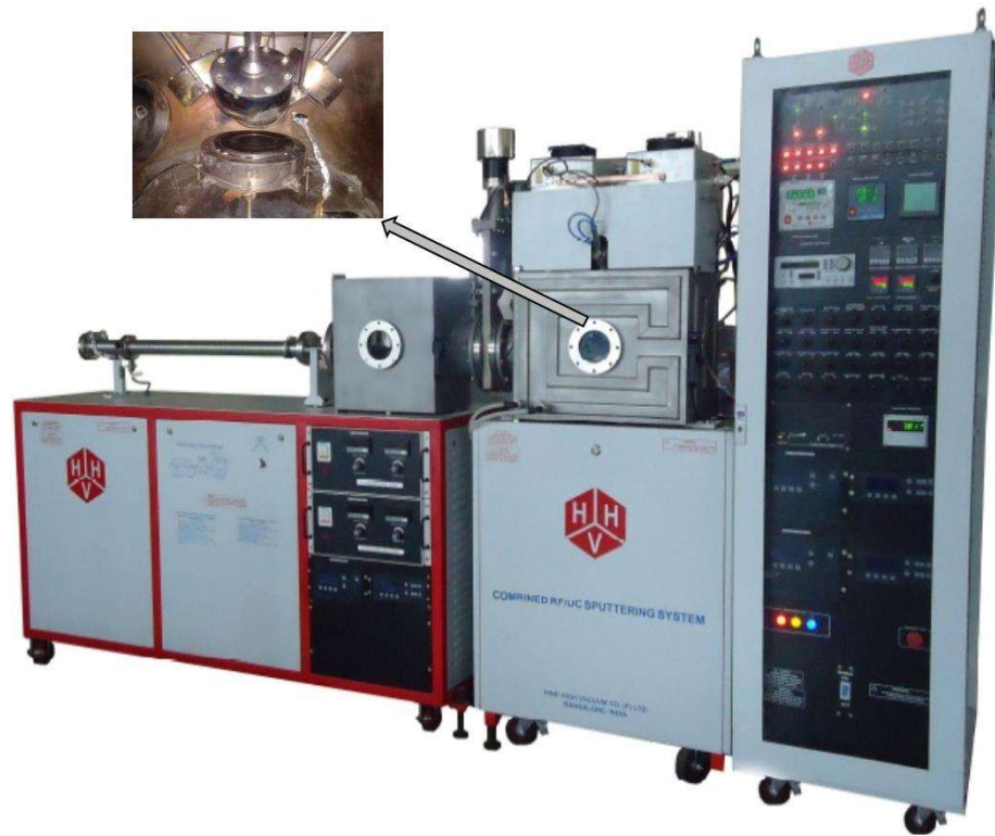
Figure 2.2: Experimental setup of RF sputtering (Hind High Vacuum combined RF/DC Sputtering System)
