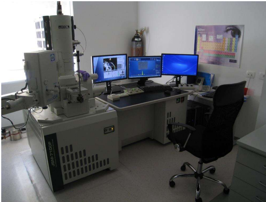
Figure 2.12: JEOL JSM-7100F FESEM instrument (Source: University of Nova Gorica, Slovenia / Material Research Lab.)
