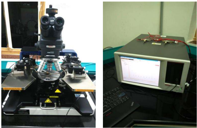
Figure 3.15: Kithley SCS 4200 electrical measurement systems
