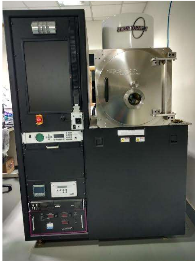
Figure 3.7: Thermal Deposition System
