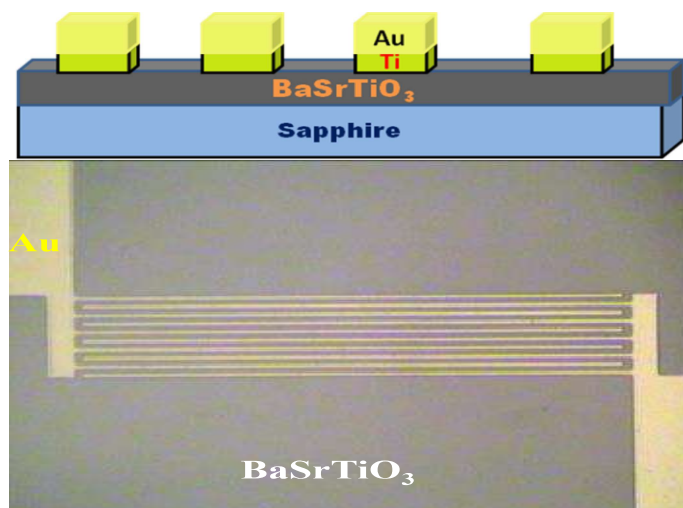
Figure 6.1: Schematic cross-section view and optical image of gold plated IDC structured Device.
