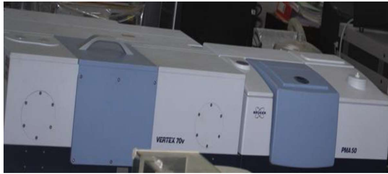
Figure 3.4 : Bruker FTIR spectrometer vertex 70v in our lab used to collect the reflectance spectra of spectrally selective absorbers
