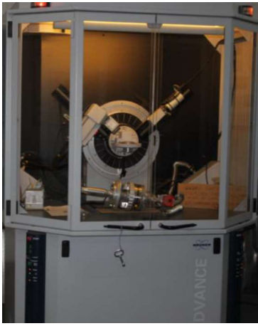
Figure 3.1 : D8 advance powder X-ray diffractometer installed at IIT Jodhpur
