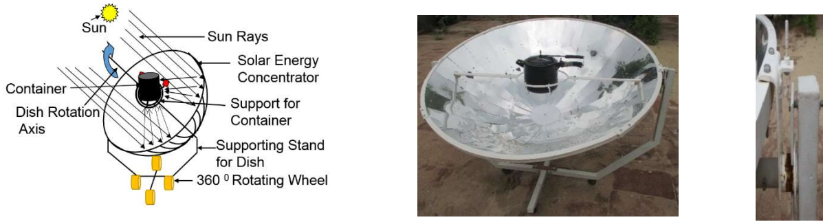
Figure 7.1: Schematic scheme (left) and real photograph (right) of dish solar energy concentrator with a container painted by black paint and kept at the focal point of dish. The rightmost photograph represents the arrangement of shadow mechanism to keep parabolic dish in normal direction to the Sun
