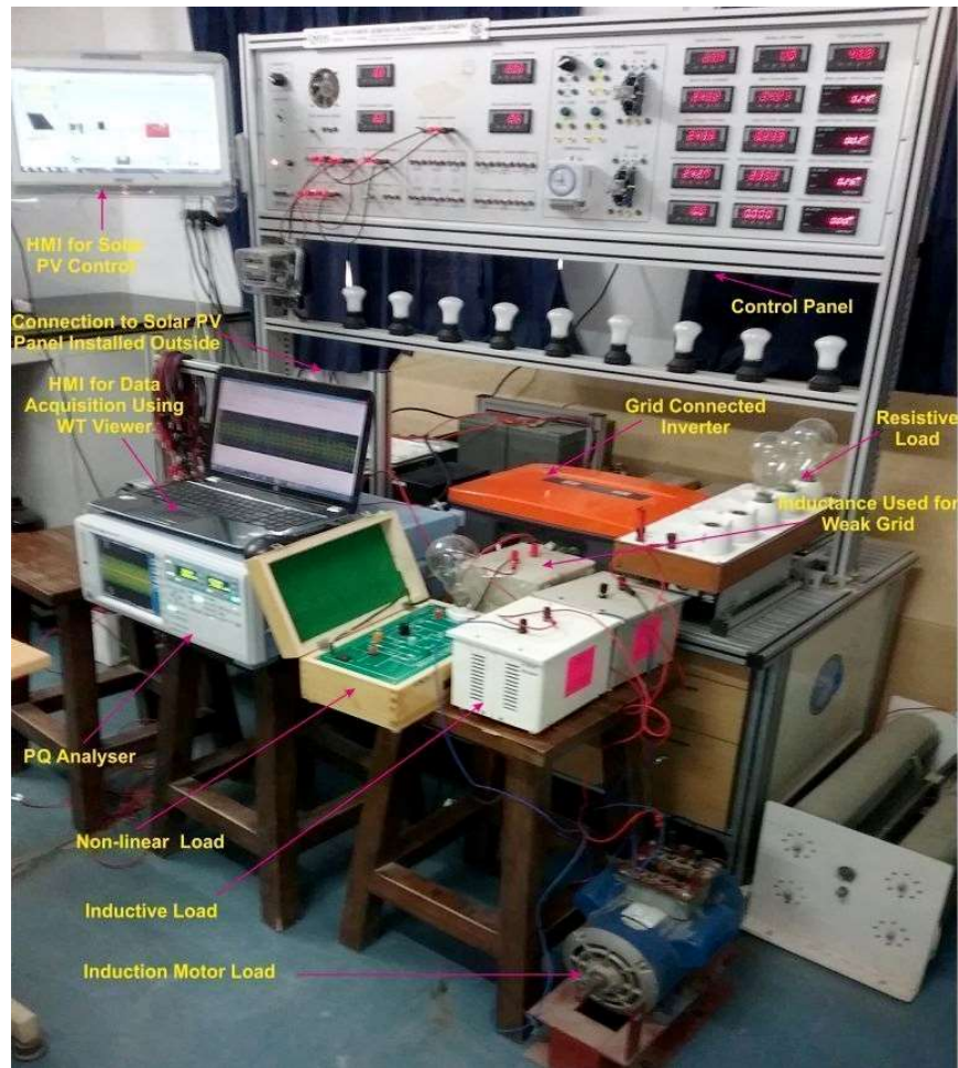
Figure 4.10 : Experimental set-up of power quality measurement with solar PV system
