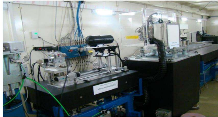
Figure 3-11 : MicroCT instrument at BL-4 RRCAT Indore
