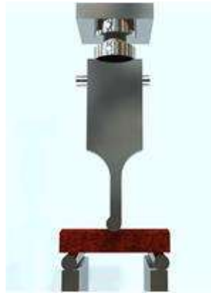
Figure 3-13 : Horizontal placement of ceramic sample over three points [Source: Plappally et al. , 2011]
