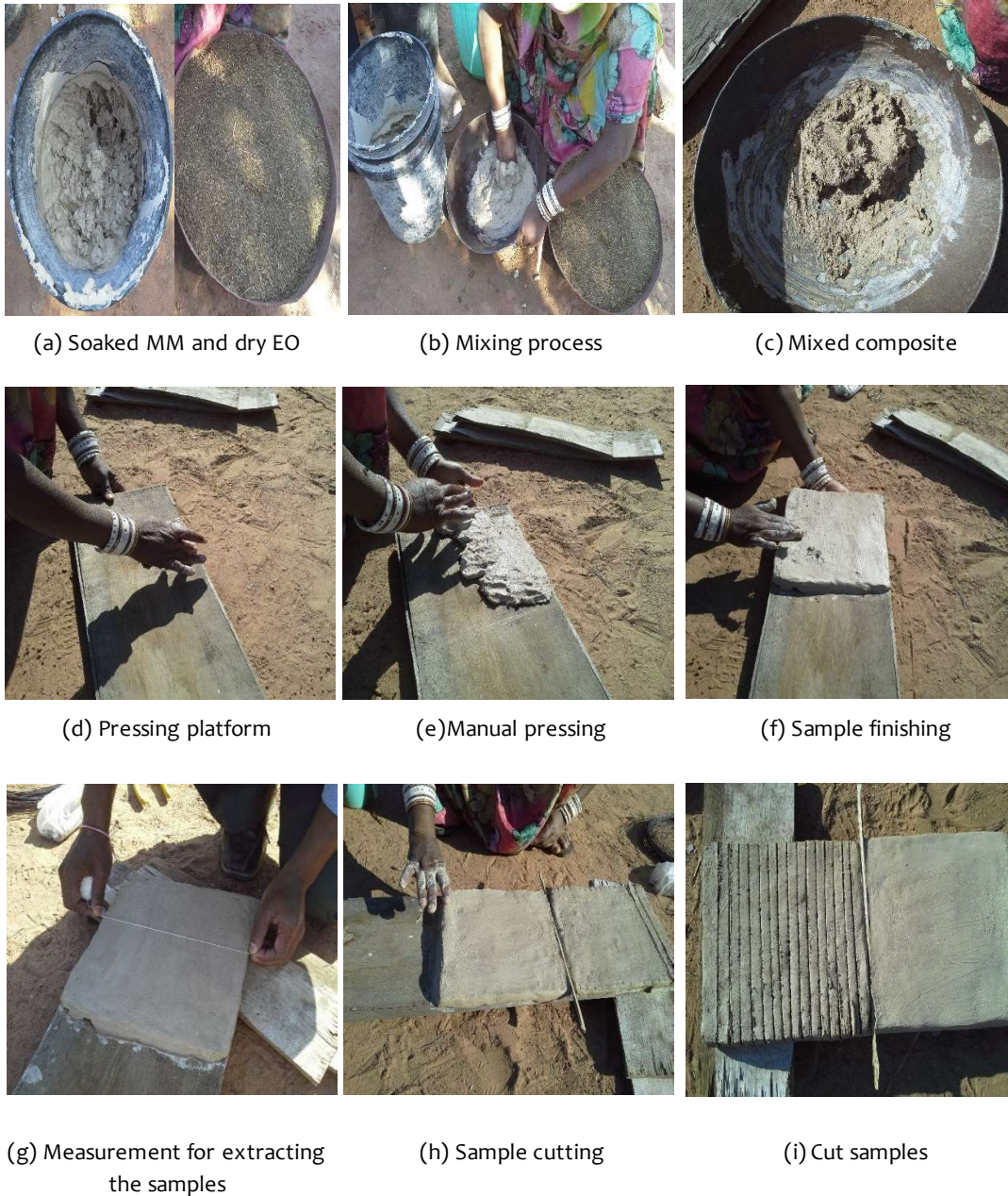
Figure 3.3: The procedure of making the MM-EO mixture and its composite samples
