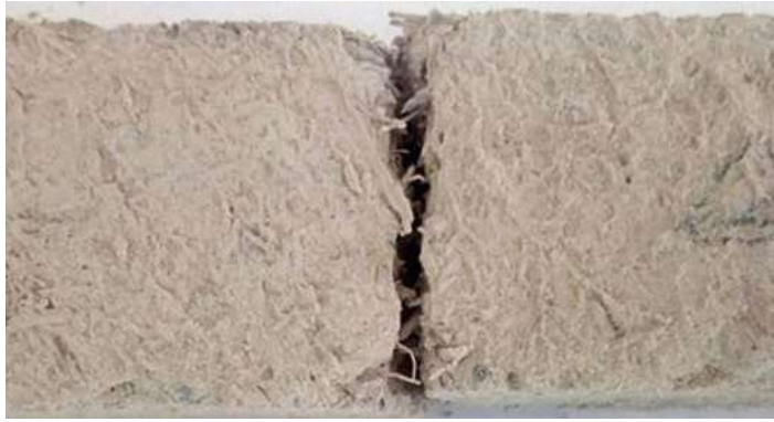
Figure 3.20: The fractured M5E5 specimen and the crack surfaces with protruding cellulosic fibers
