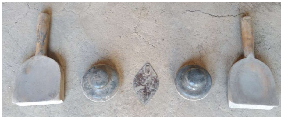
Figure 4.6: Traditional paddling tools used in Indian pottery manufacturing
