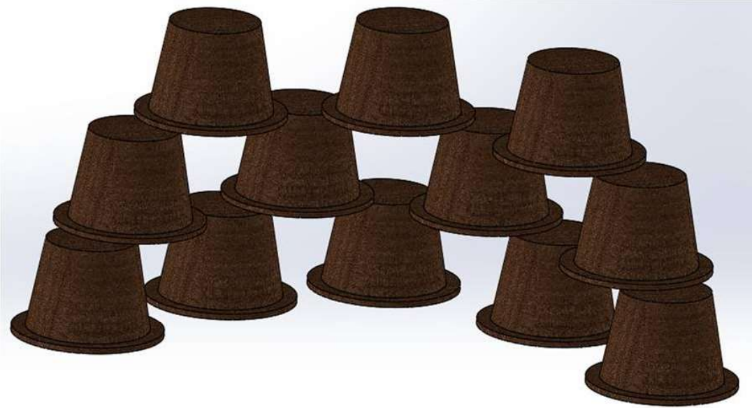
Figure 5.5: The geometrical arrangement of filter greenware (G-filter) within the up-draught furnace (Solidworks, 2015, IIT Jodhpur License)
