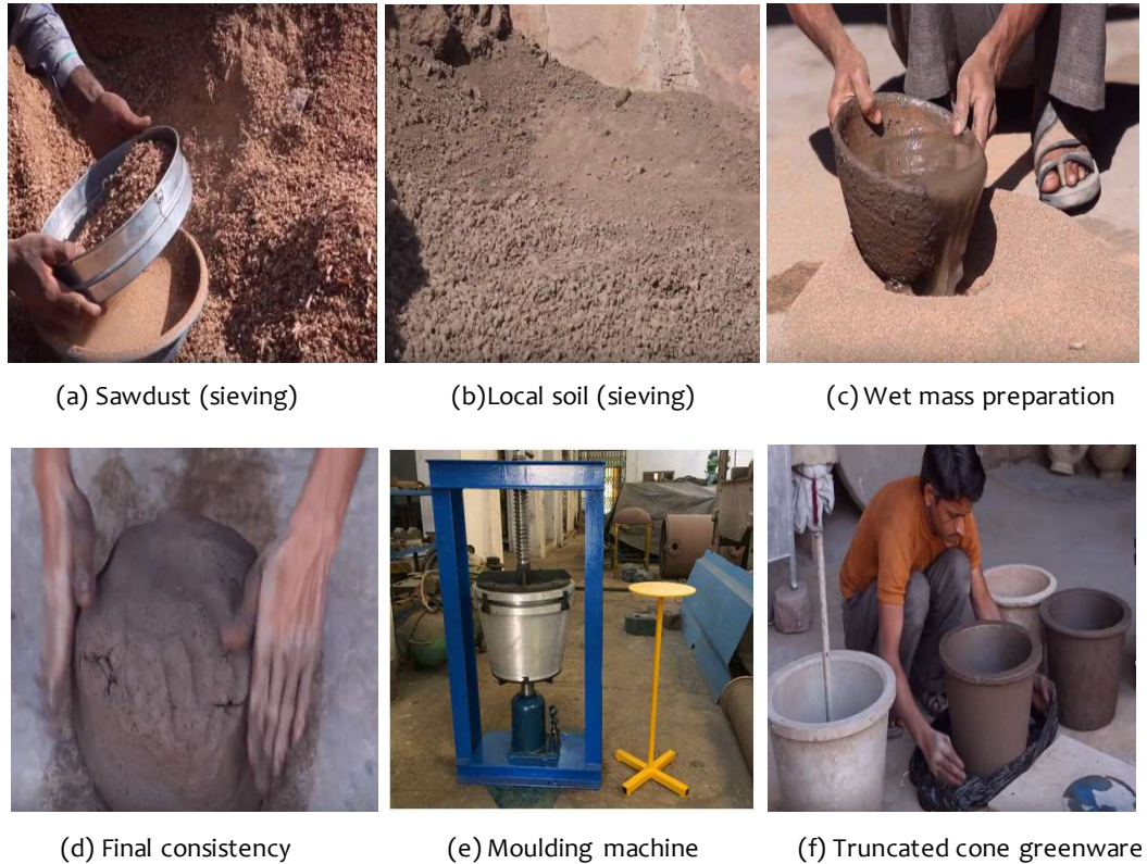
Figure 5.4: G-filter manufacturing steps
