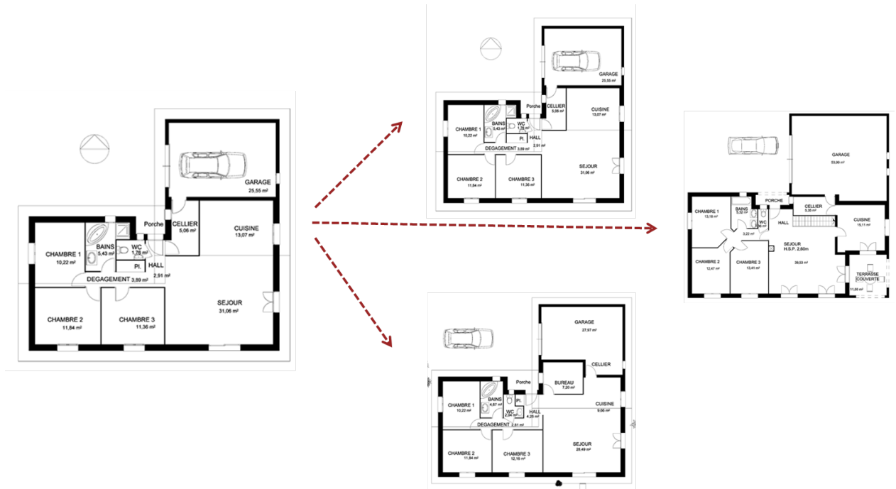
Figure 1.6. : Retrieval in floor plans by extracting meaningful content and looking for similarity across floor plan databases.
