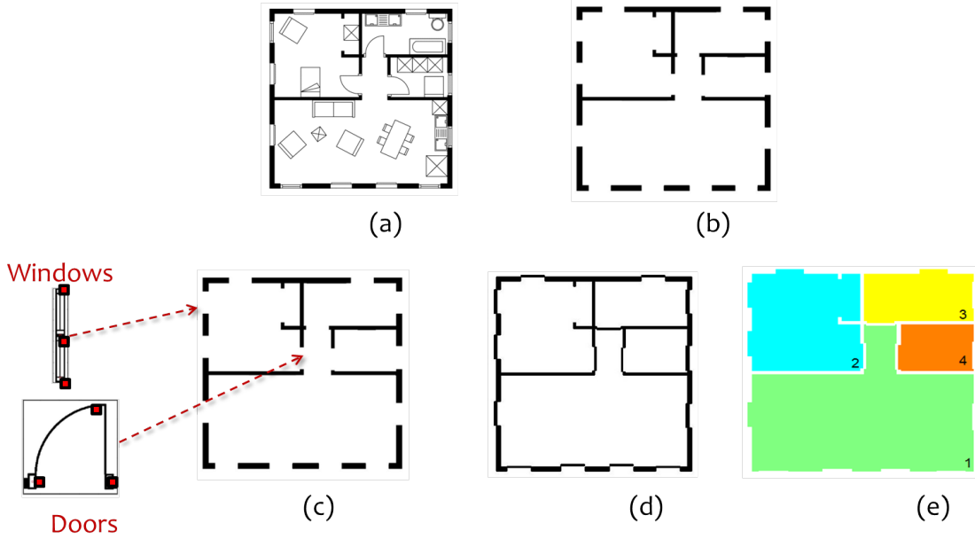
Figure 3.2. : Various stages of structural and semantic analysis on an image from SESYD dataset [Delalandre et al. , 2010a]: (a) unsegmented layout, results of (b) morphological operation and wall, boundary extraction, (c) Detection of doors and windows (d) Closing gaps in walls and (e) labelling and segmenting the room structure
