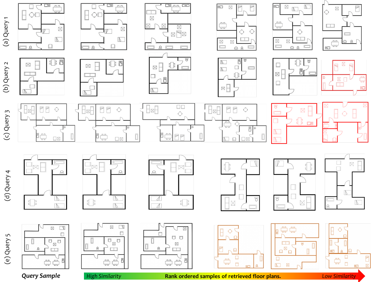
Figure 4.9. : Rank ordered retrieval result of the proposed framework for five different query floor plans from the ROBIN dataset. Here, top five rank ordered floor plans are shown for each query.
