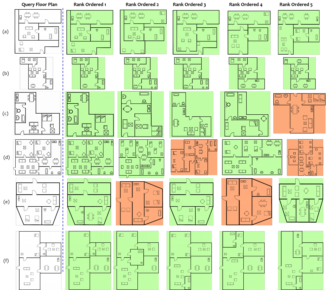
Figure 5.10. : Retrieval results for four different query architectural floor plans taken from the ROBIN dataset. Note that the floor plans highlighted in red are incorrectly retrieved as global layout shape differs from query.
