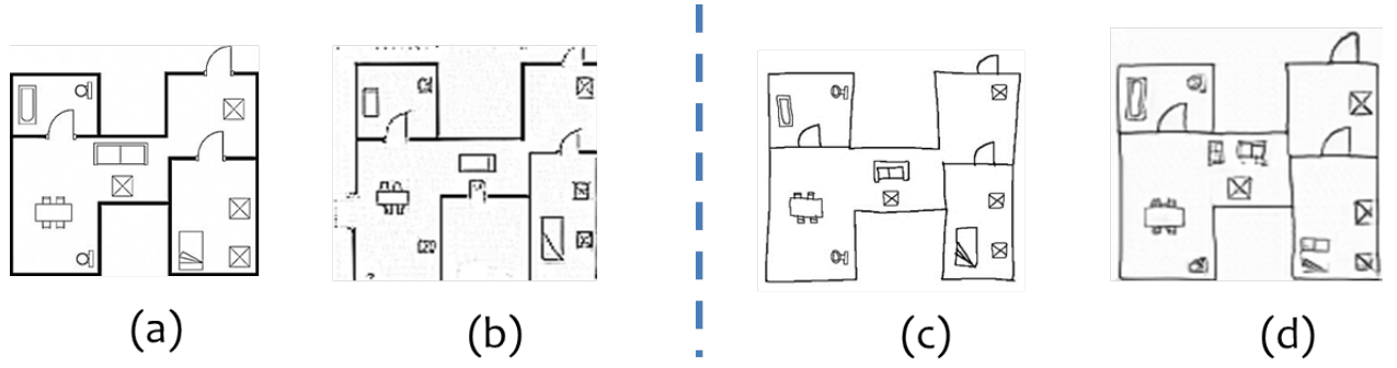
Figure 6.3. : Comparing the original sketches/images with outputs generated from Cyclic GAN. (a) Original floor image from ROBIN dataset. (b) Generated floor plan image using Cyclic GAN. (c) Original floor plan sketch from S-ROBIN dataset. (d) Generated floor plan sketch using Cyclic GAN. Kindly note the quality of generated sketches is better than that of generated images.
