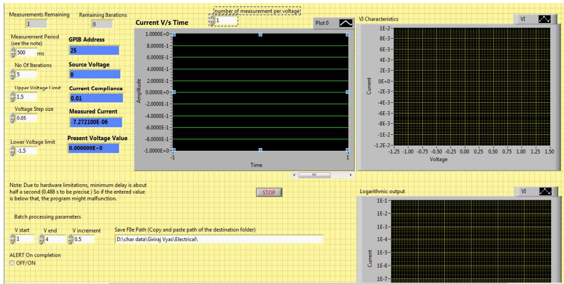
Figure 2.9: Front panel of Voltage Sweep VI with batch processing and Logarithmic output display,
