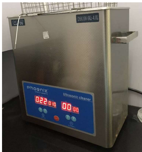
Figure 2.1: The DSA100-SK2-4.0L Ultrasonic cleaner from Phoenix instrument used in the current study.
