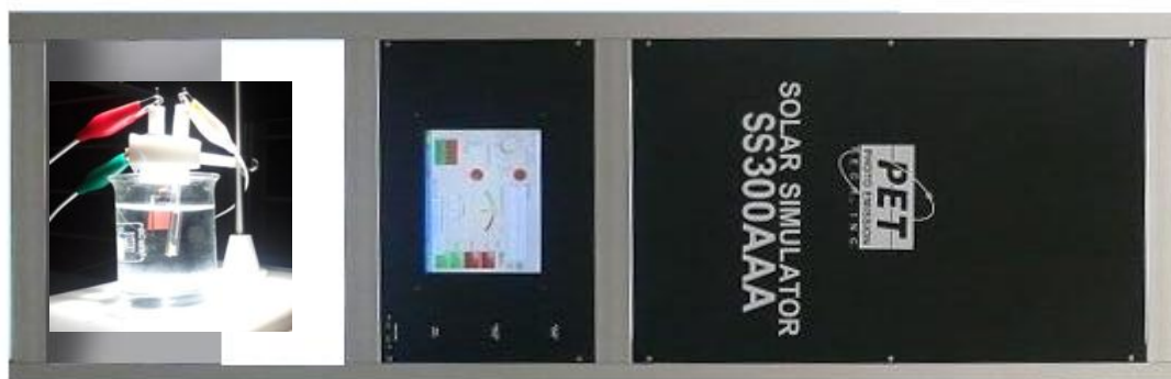
Figure 2.11: I-V measurement under 100 \text{ W/m}^2 solar simulator radiation
