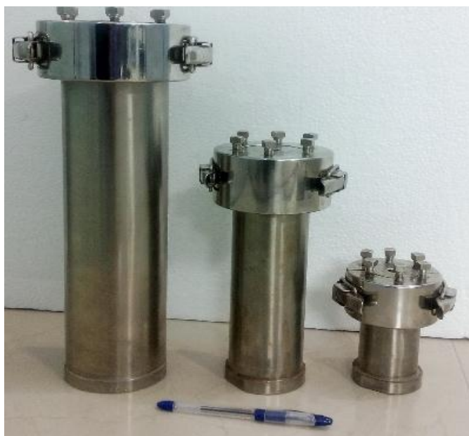
Figure 2.2: Hydrothermal reaction vessel of 100 mL, 250 mL and 800 mL capacity
