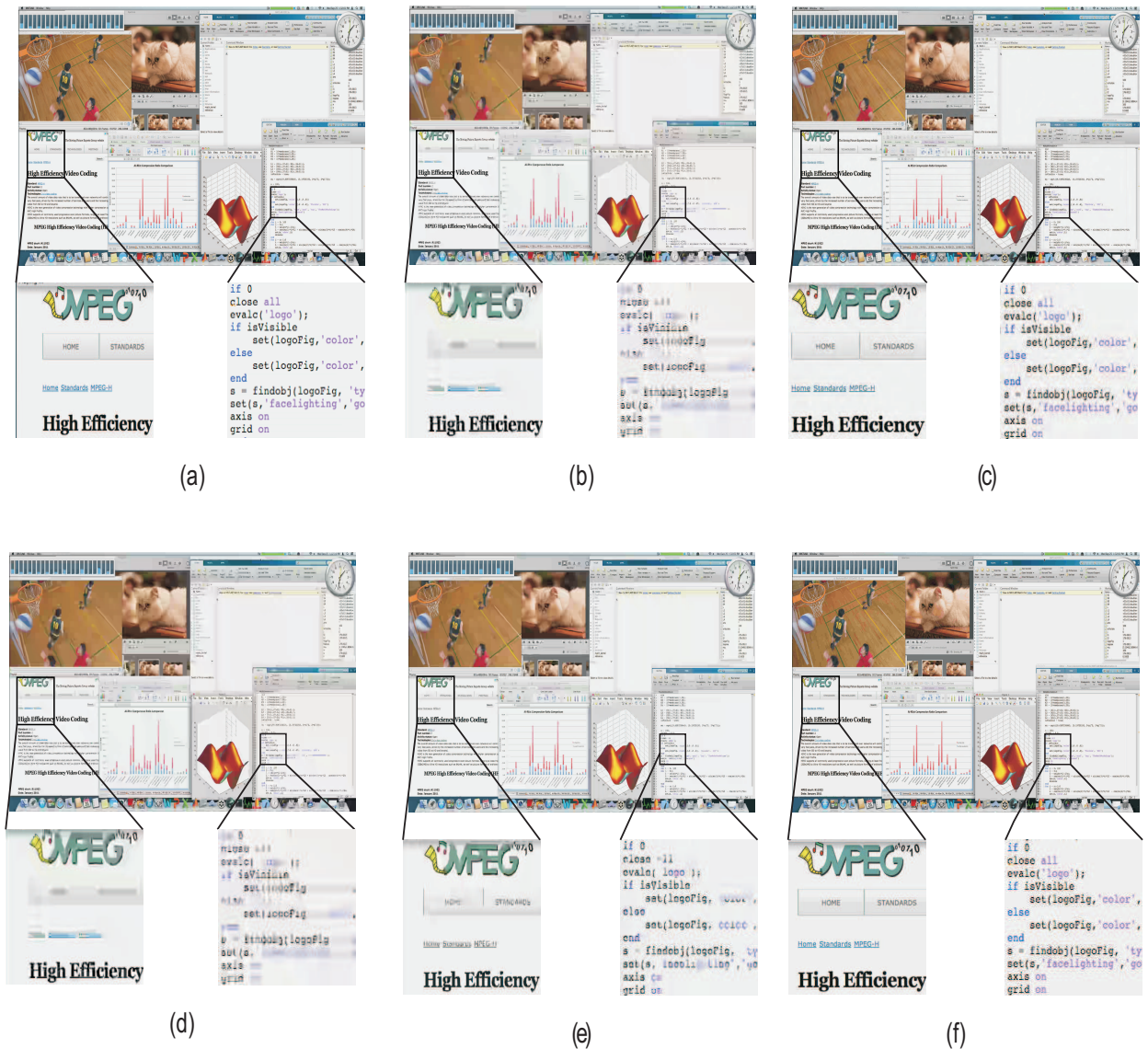
Figure 3.8 : Comparison on quality of the reconstructed image at 0.8 bpp by using different methods (a) Original SCI, (b) After applying JPEG [Wallace, 1992], (c) After applying JPEG 2000 [Skodras et al. , 2001], (d) After applying HEVC [Sullivan et al. , 2012], (e) After applying HEVC for SCC [Xu et al. , 2016], and (f) After applying the proposed method.
