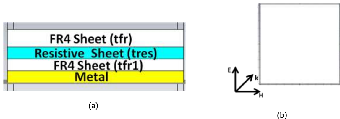
Figure 6- 1: (a) Side and (b) top view of TLMA along with wave vector, electric and magnetic field directions
