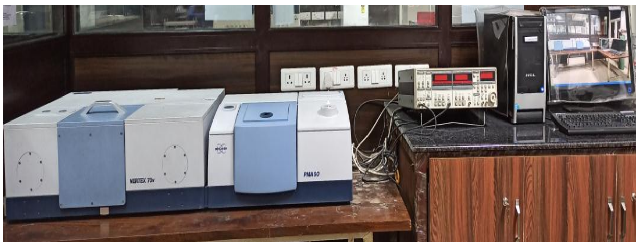
Figure 3.8 Optical image of FTIR spectrometer used for reflectance measurement at IIT Jodhpur
