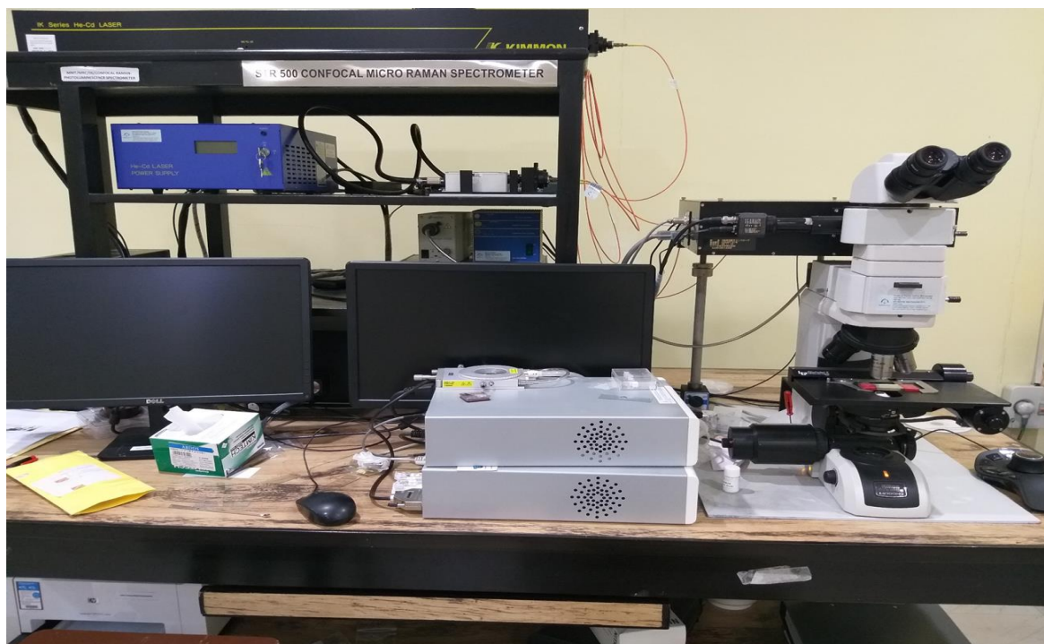
Figure 2.14: Instrument setup of Raman spectroscopy. (Courtesy: Material Research Centre, MNIT Jaipur)
