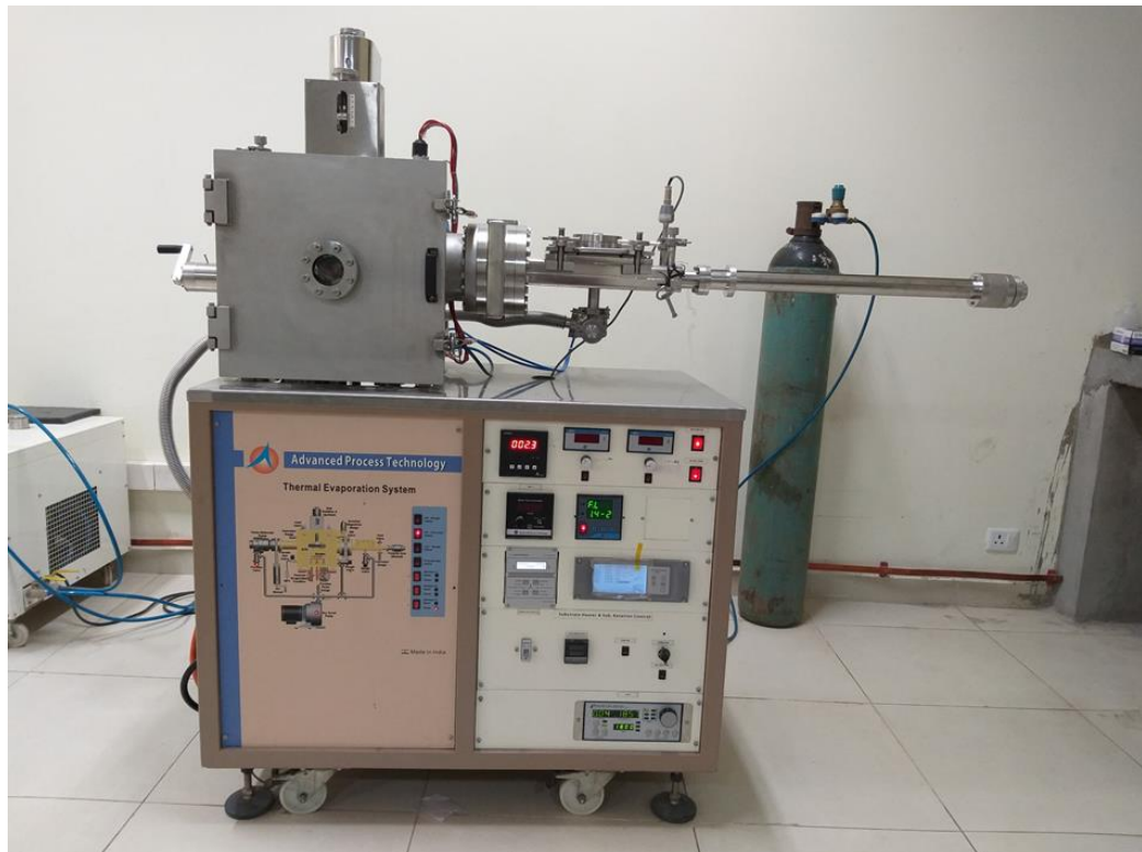
Figure 2.23: Photograph of thermal evaporation system.
