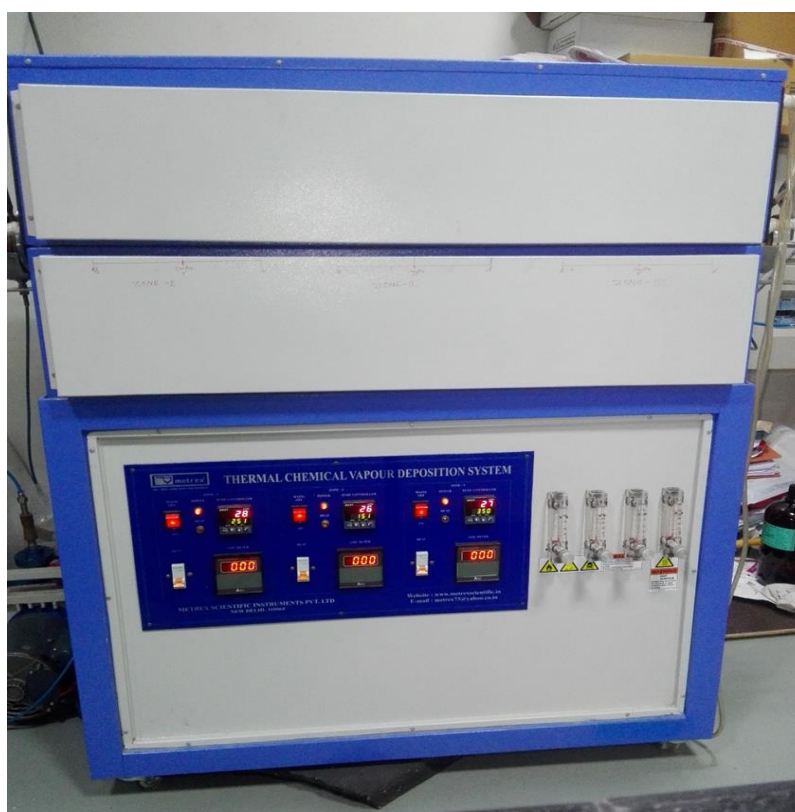
Figure 2.4: Optical image of chemical vapor deposition (CVD) system.
