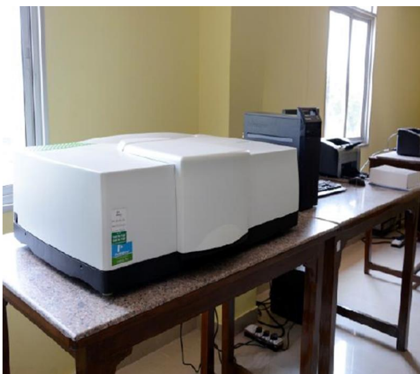
Figure 2.15: Experimental setup of UV/Vis spectrophotometer.
