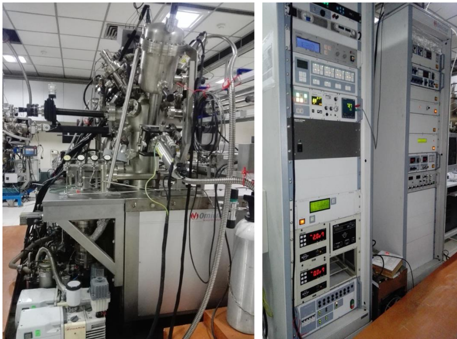
Figure 2.20: Photograph of the X-ray photoelectron spectroscopy system, which is used for this thesis work. (Courtesy: Thin Film Devices & Metrology Section, CSIR-NPL New Delhi)
