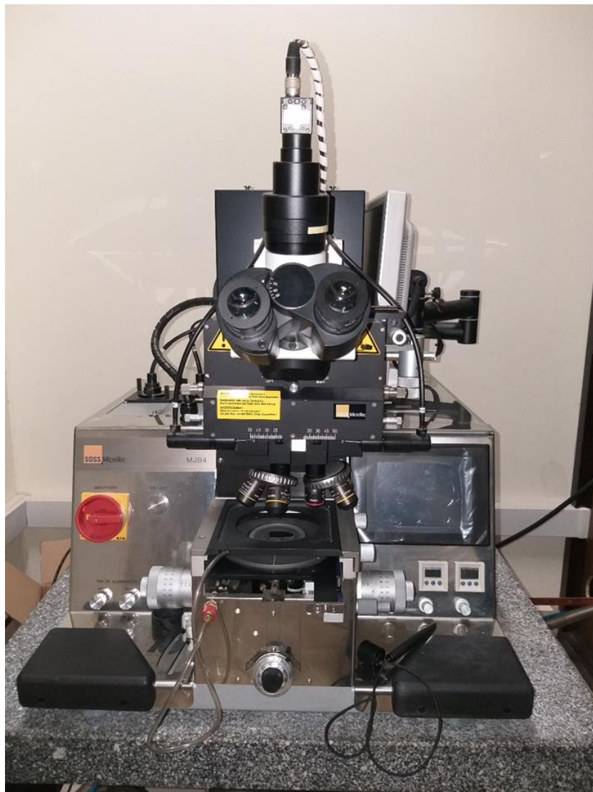
Figure 2.26: Photograph of Mask Aligner: Optical Lithography.
