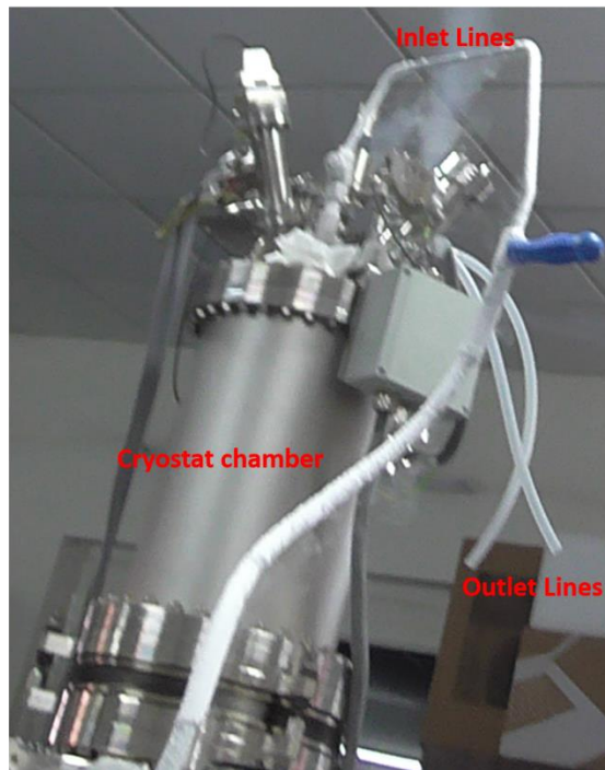
Fig 2.8 Schematic representation of cryostat and image of cryostat mounted on top of LT-STM while transferring liquid nitrogen from Dewar.
