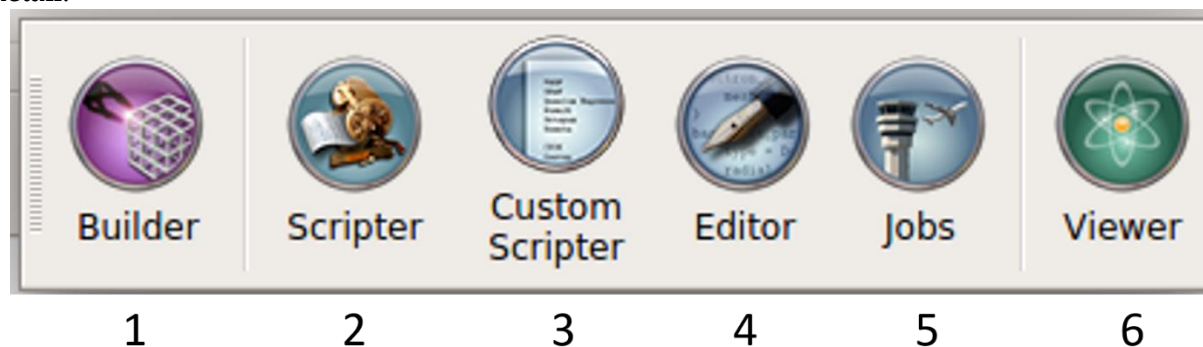
Fig 3.2 VNL tool is divided into three main sections: geometry, Scripting and analysis. 1 is responsible for defining the exact geometry of the atoms. 2, 3, 4 and 5 corresponds to scripting section and 6 corresponds to data evaluation section.
