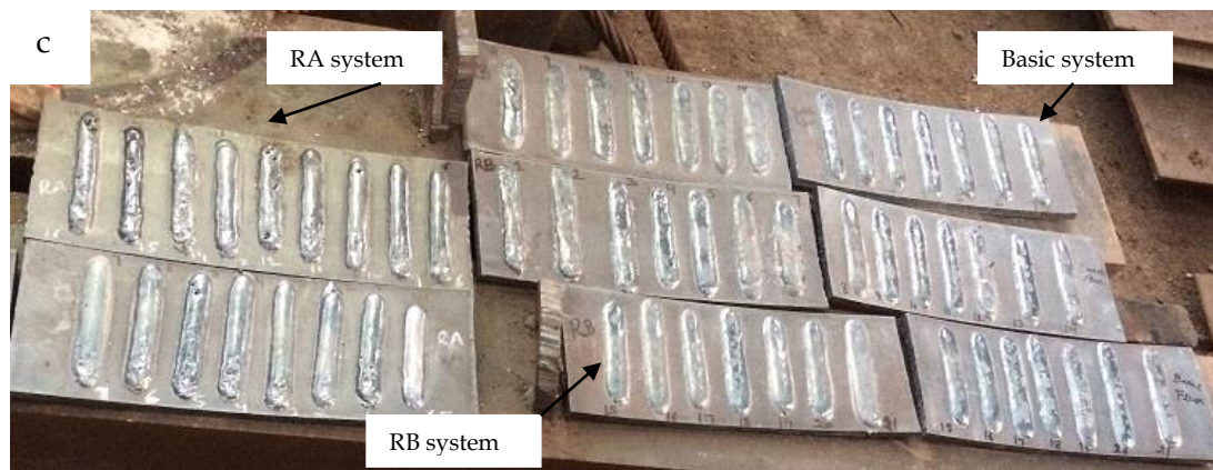
Figure 4.7: Steps of multi-pass bead on plate weld deposits experimentation using SAW machine.
