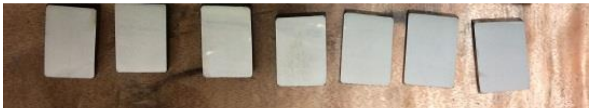
Figure 4.13: Specimens for microhardness testing of weld and HAZ
