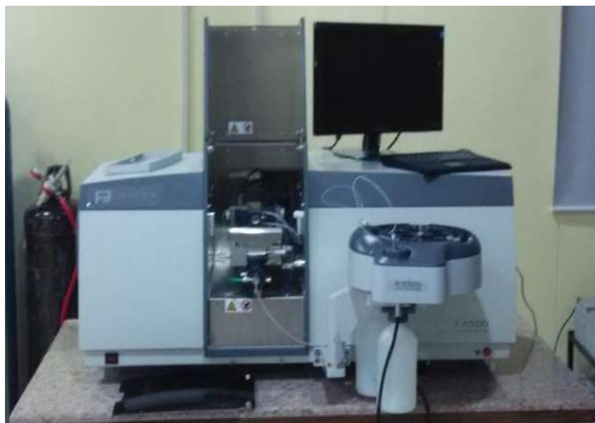
Figure 3.21: Atomic Absorption Spectroscopy system for elemental analysis of solutions (Source: MRC, MNIT Jaipur)
