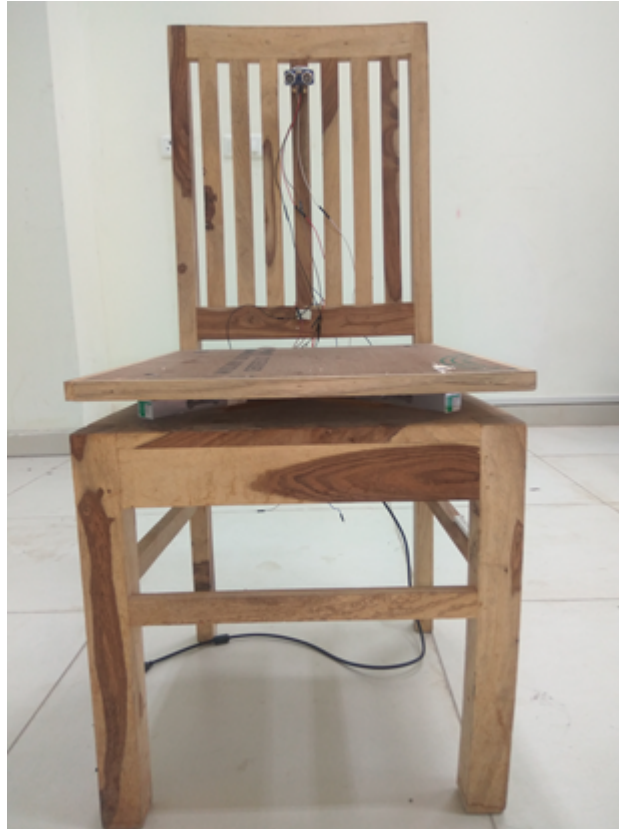
Figure 7.7 : Chair with Ultrasonic sensor
