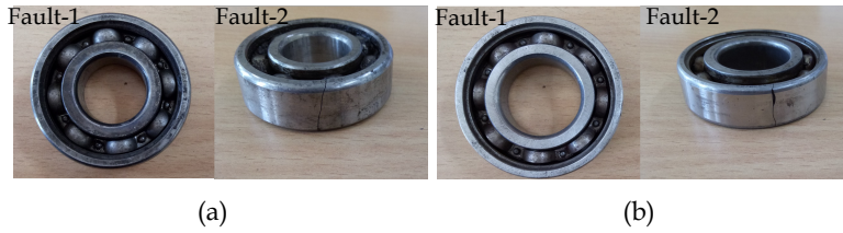
Figure 4.15 : Bearings with Fault-1: Ball fault and Fault-2: Outerrace fault at (a) fan-end and (b) driving-end of the motor
