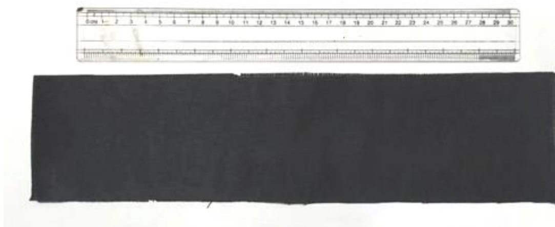
Figure 5.2: Photograph of carbon cloth coated with Ni-Co ink ( 35 \times 10 \text{ cm}^2 ) demonstrating scalability of the synthesis process.
