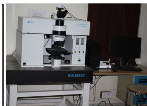
Figure 4.7: (a) Schematic for optical design of Raman Microscope (Source: Schrader, 1995) (b) Nomadic Raman spectrophotometer (Make: BaySpec, USA)
