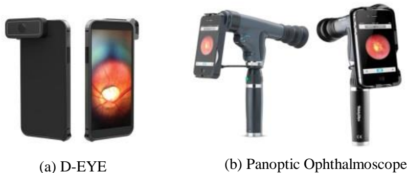
Figure 1.2 : Advanced fundus image acquisition devices: (a) D-EYE, (b) Panoptic Ophthalmoscope. Image Credits: D-EYE [HOSPEQ, 2020], and Panoptic Ophthalmoscope [EYEWIRE.News, 2020]
