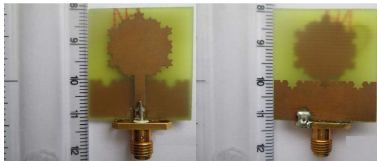
Figure 3.61: Fabricated prototype of the antenna (a) Top view and (b) Bottom view
