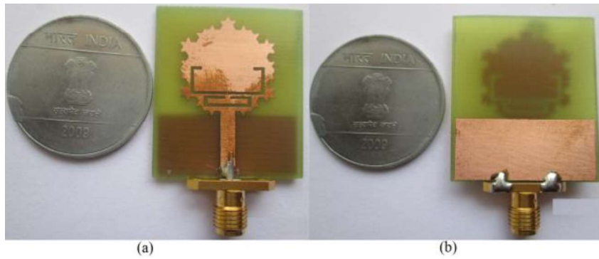
Figure 4.14: Photograph of the fabricated antenna (a) top view and (b) bottom view
