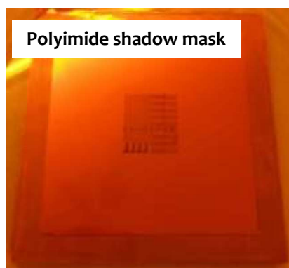
Figure 3.5 :Photograph of a Polyimide Shadow Mask Used in Deposition Process
