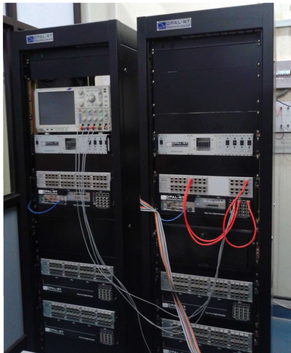
Figure 4.3 : An image of OPAL-RT digital simulator used for real-time simulation studies
